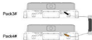
Figure 6-3 Insert Fuse Plugs into PACK Bases
